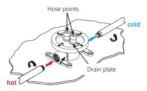
8. Screw the copper pipes into the base of the mixer body and then attach the chrome shaft to the mixer body. Finally, attach the shroud and fixing bracket to the chrome shaft.
