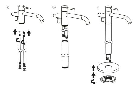
9. Push the copper pipes into the hot and cold inlets on the water inlet collar. **NOTE:** the hot supply pipe is on the left and the cold supply pipe is on the right. Next, secure the water inlet collar to the fixing bracket using the 4 x 16mm screws that were removed from the drain plate in step 7.
