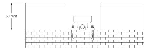
5. Once you have set the correct recess in your floor, use an allen key to remove the 4 x 22mm screws that hold the mortar guard onto the fixing seat and remove the mortar guard. Keep the screws to one side.
