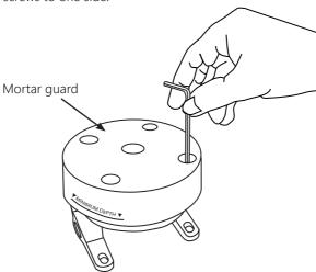
6. Mark the positions of the 4 fixing points in the fixing seat. Drill holes and use the floor fixing bolts to secure the fixing seat in position. **NOTE:** the fixing seat can be fixed in any orientation inside your recess as the final fix parts are fully adjustable.
